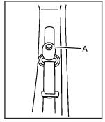
To move it down, push the release button (A) and move the height adjuster to the desired position. You can move the adjuster up just by pushing up on the shoulder belt guide.
